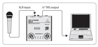
Fig. 3.2: Connection of the MIC200 and the soundcard of your PC
